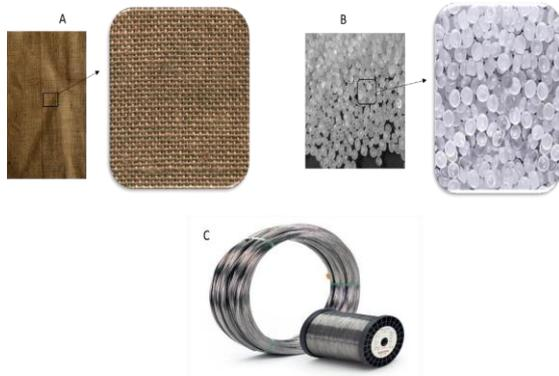
**Gambar 1. (a) Serat Jute, (b) Polypropylene, (c) Kawat Nikelin**
