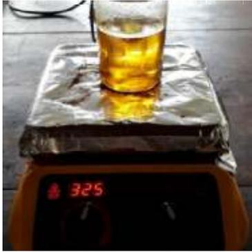
**Gambar 3 Proses heat treatment getah pinus**
