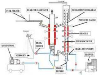
Gambar 1. Skematik dual reactor fluidized bed (DRFB)
