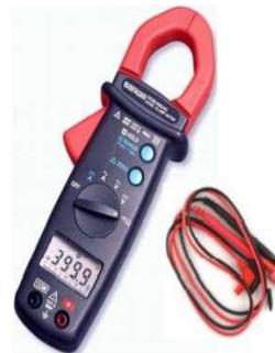
**Gambar 3.3 Alat ukur Tang Meter**
