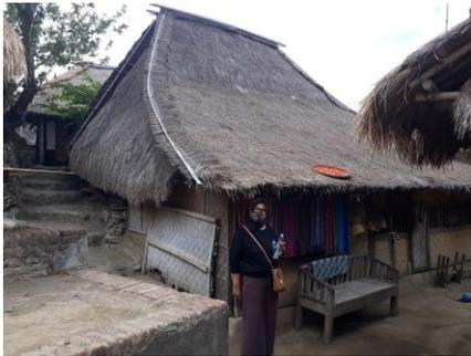
Figure 5. Building materials: alang-alang/thatched roof and bamboo walls
